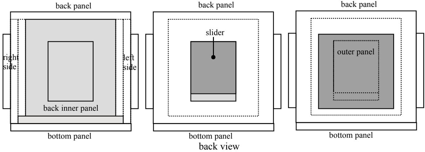
Move the bottom slider forward, and drop the back, left and right sliders. Place the top inner panel in position on top of the left and right inner panels. Bring it forward so that the angled cuts meet. Now raise the back, left and right sliders to lock the top inner panel into place.
