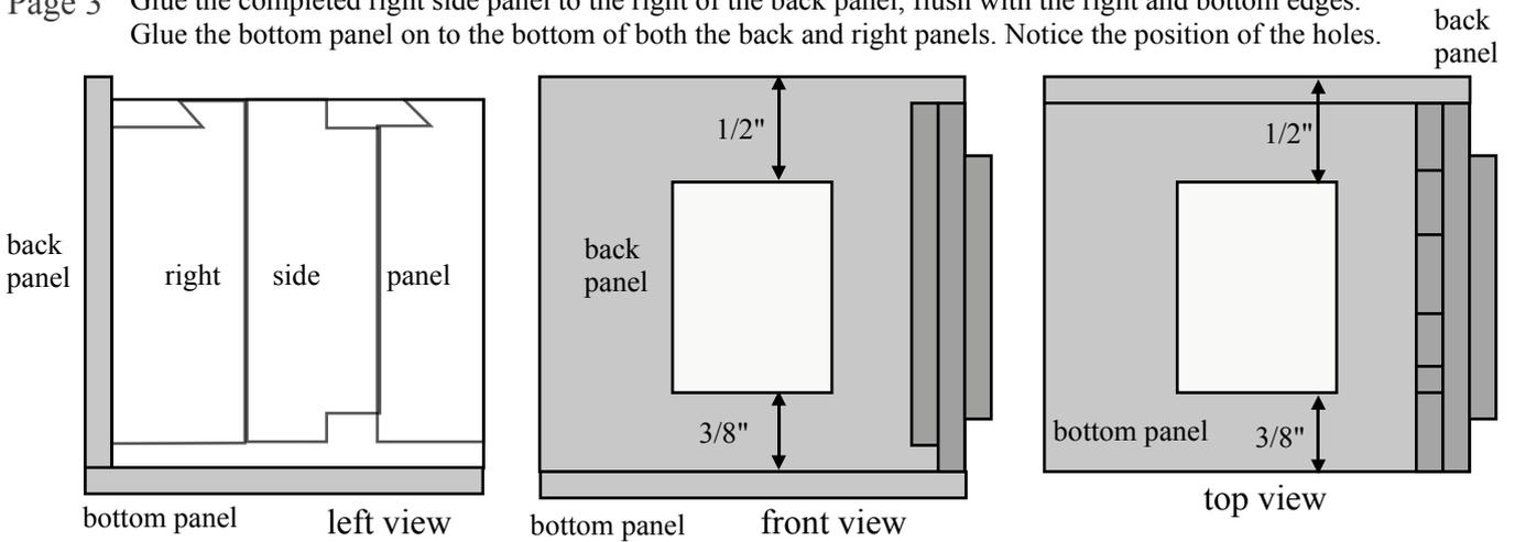
Do the same with the completed left side panel, glued to the left side of the back and bottom panels
