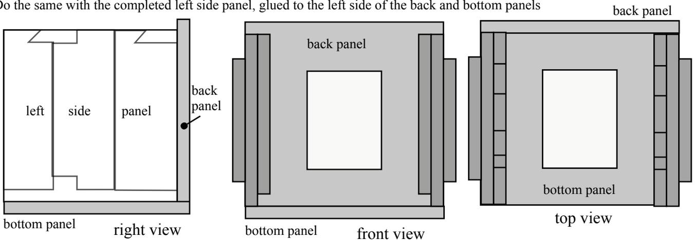
Slide the bottom inner panel beneath the left and right inner panels, all the way to the back.
