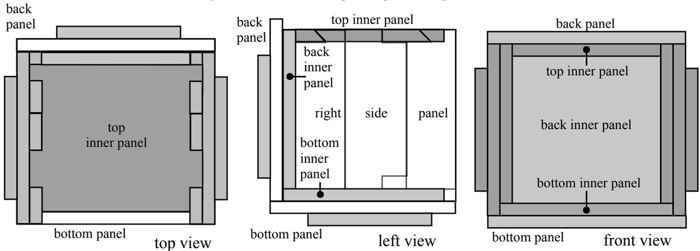
Place the top panel onto the top inner panel. Notice that it will overhang the front edges of the left and right sides. Do NOT glue it! Glue a slider onto the top inner panel through the hole. The slider should be at the front of the hole. Glue an outer panel to the slider. It should be in the middle of the top.
