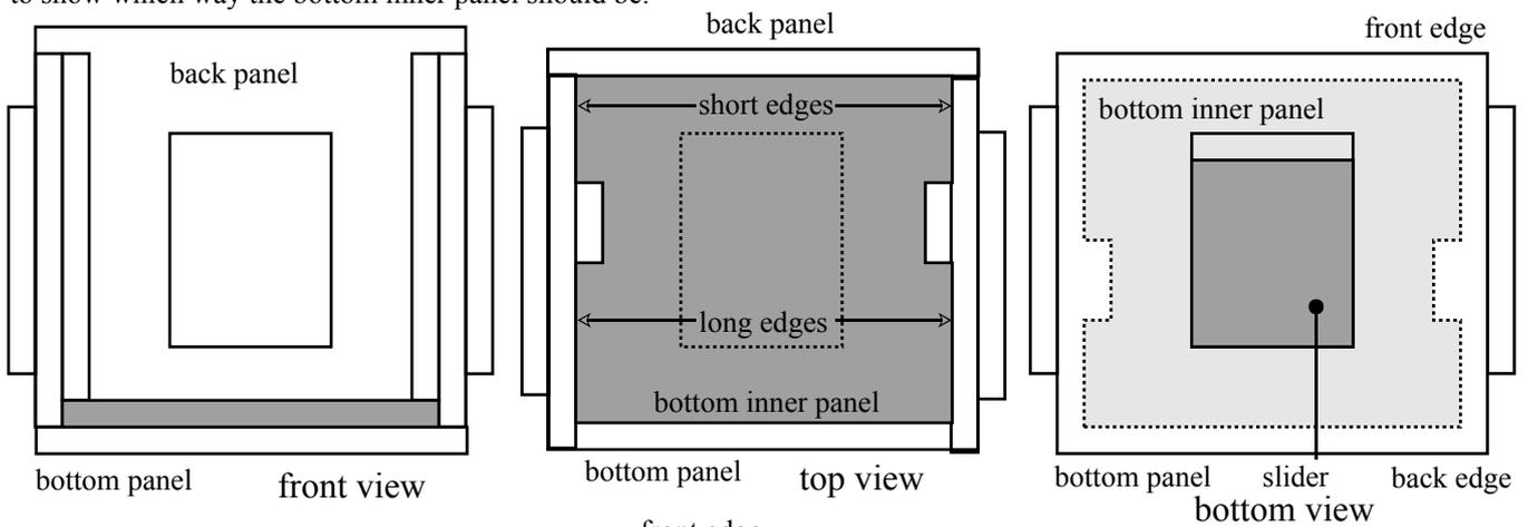
If the bottom inner panel is in the correct way round, when you move the bottom slider forward, you should be able to drop the left and right sliders. The middle panels on both sides (right 2 and left 2) should drop into the slots in the bottom inner panel. Check this before the bottom inner panel is glued into place!
