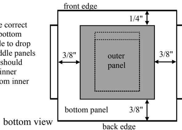
Glue an outer panel to the slider. Notice the position of the panel. When the glue has set, check that the outer panel will move, taking the slider and bottom inner panel with it.
