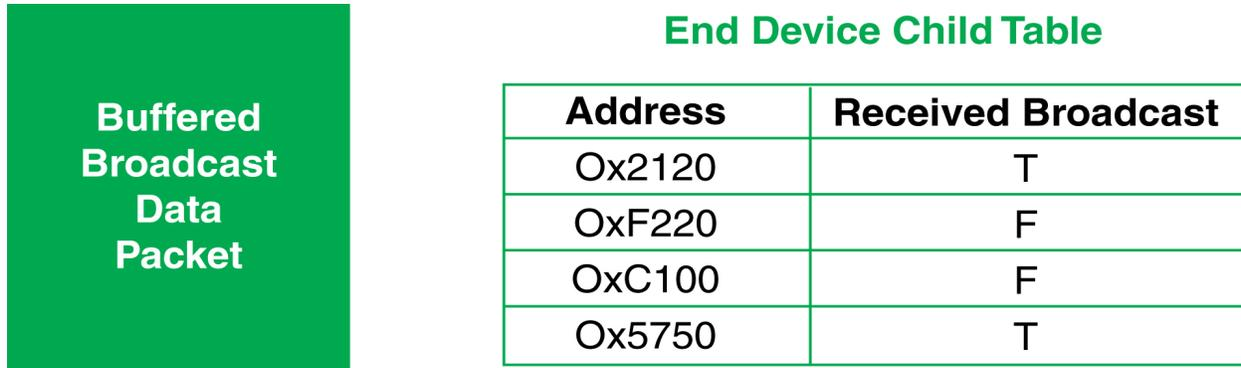
When an end device sends data to its parent that is destined for a remote device in the network, the parent buffers the data packet until it can establish a route to the destination. The parent may perform a route or 16-bit address discovery in behalf of its end device children. Once a route is established, the parent sends the data transmission to the remote device.
