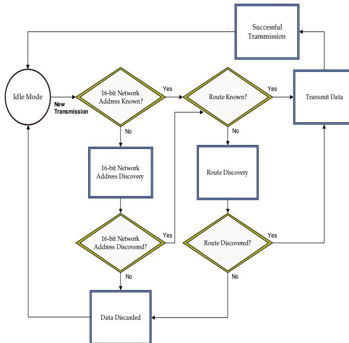
When data is transmitted from one node to another, a network-level acknowledgement is transmitted back across the established route to the source node. This acknowledgement packet indicates to the source node that the data packet was received by the destination node. If a network acknowledgement is not received, the source node will re-transmit the data.
