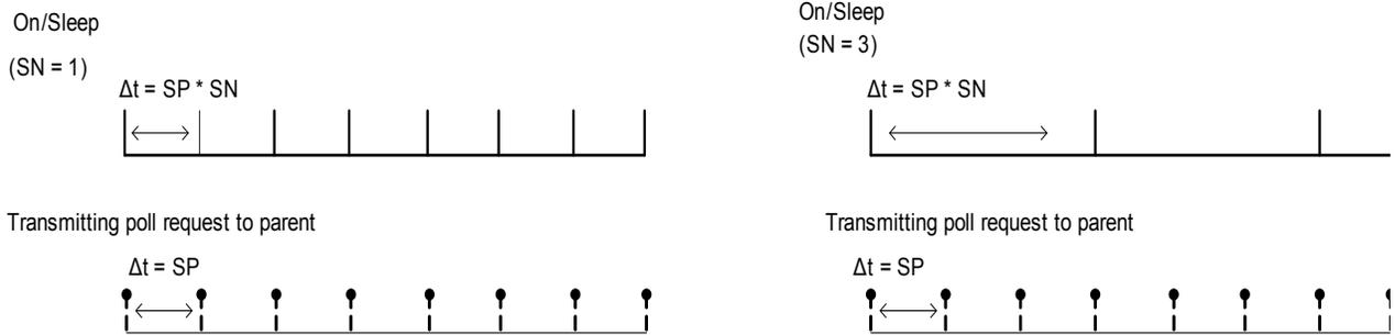
**Setting SN > 1 allows the XBee to silently poll for data without asserting On /Sleep. If RF data is received when polling, On/Sleep will immediately assert .**
