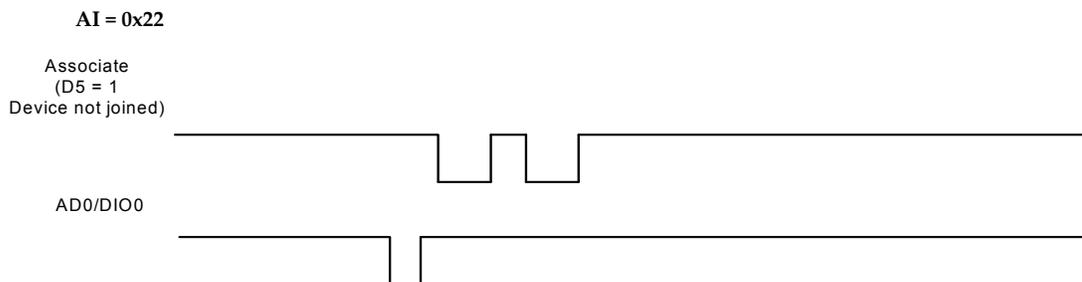
**A single commissioning button press when the device has not joined a network that causes the associate pin to blink to indicate the AI Code where: AI = # blinks + 0x20. In this example, AI = 0x22.**
