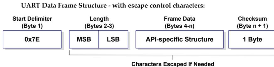
MSB = Most Significant Byte, LSB = Least Significant Byte
