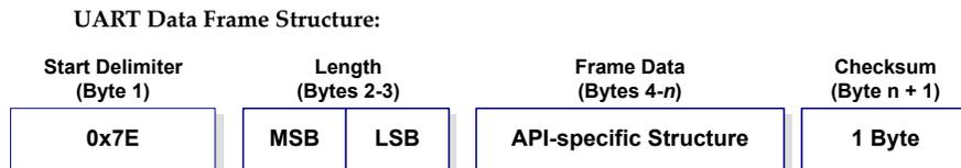
MSB = Most Significant Byte, LSB = Least Significant Byte
