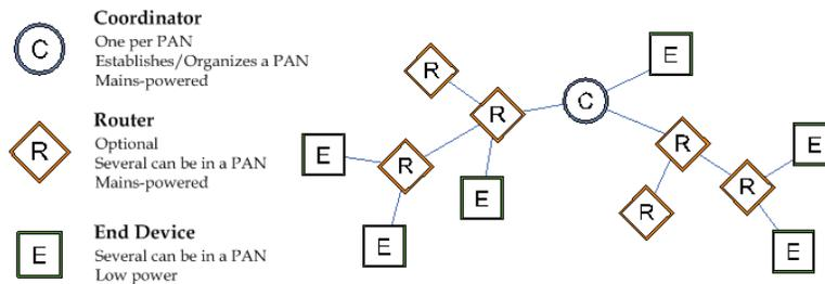
In ZigBee networks, the coordinator must select a PAN ID (64-bit and 16-bit) and channel to start a network. After that, it behaves essentially like a router. The coordinator and routers can allow other devices to join the network and can route data.
