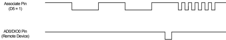
**A single button press on a remote device causes a broadcast node identification transmission to be sent. All devices that receive this transmission blink their associate pin rapidly for one second if the associate LED functionality is enabled. (D5 = 1)**
