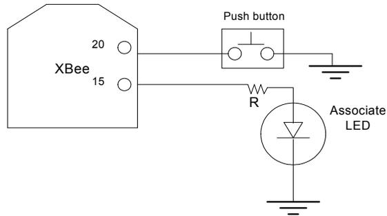
**A pushbutton and an LED can be connected to module pins 20 and 15 respectively to support the commissioning pushbutton and associate LED functionalities.**
