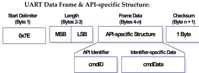
The cmdID frame (API-identifier) indicates which API messages will be contained in the cmdData frame (Identifier-specific data). Note that multi-byte values are sent big endian. The XBee modules support the following API frames:
