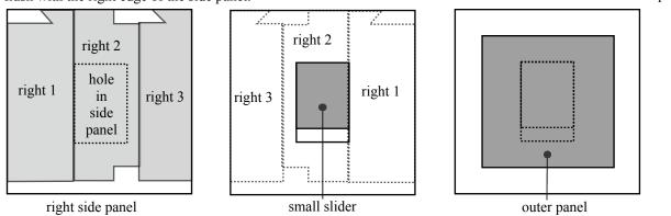
Do the same with the left side panel: this is a mirror image of the right side. When glue has set, check for movement.
