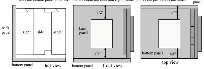
Do the same with the completed left side panel, glued to the left side of the back and bottom panels
