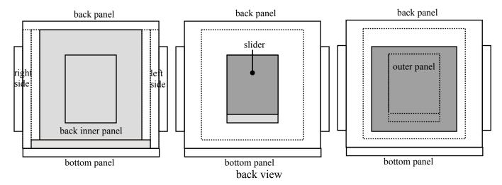
Move the bottom slider forward, and drop the back, left and right sliders. Place the top inner panel in position on top of the left and right inner panels. Bring it forward so that the angled cuts meet. Now raise the back, left and right sliders to lock the top inner panel into place.
