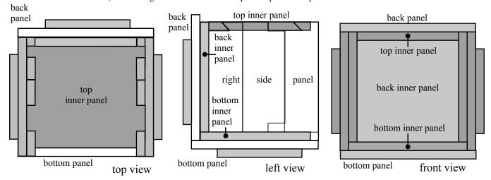
Place the top panel onto the top inner panel. Notice that it will overhang the front edges of the left and right sides. Do NOT glue it!
