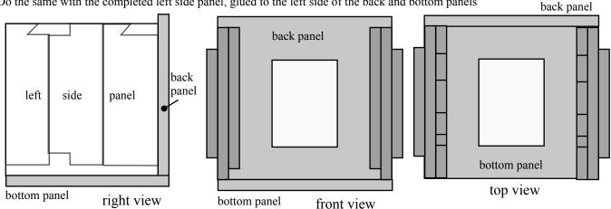
Slide the bottom inner panel beneath the left and right inner panels, all the way to the back. In this top view, the left and right inner panels are not shown, to show which way the bottom inner panel should be.
